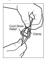
Should the power cord come loose from the cord strain relief, it can be easily reattached.
